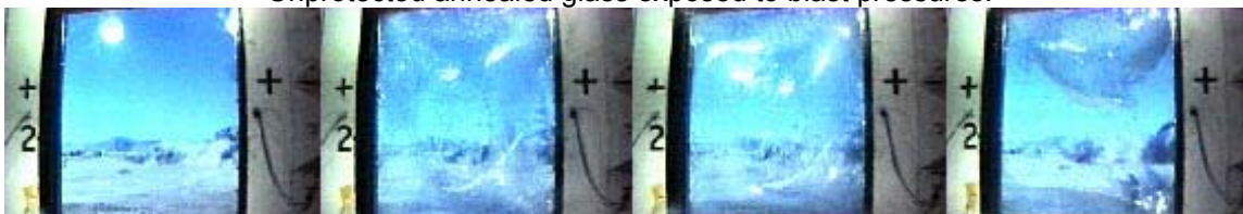
Security window film applied to annealed glass exposed to blast pressures.
