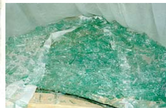
Blast Curtain pre- and post-explosion.
